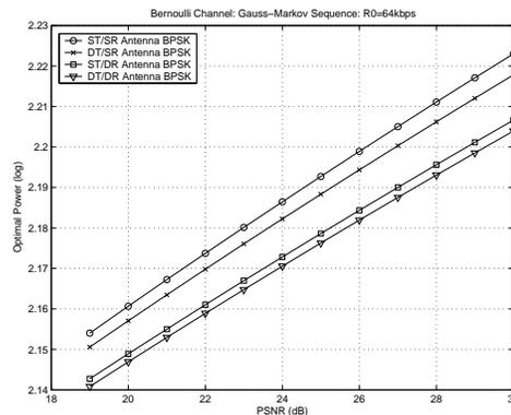
Fig. 3. BPSK plot of optimal power versus peak signal to noise ratio for single/double transmit/receive antenna systems. A Gauss-Markov source with parameter  $\rho = 0.9$  and the Bernoulli loss model have been considered.
