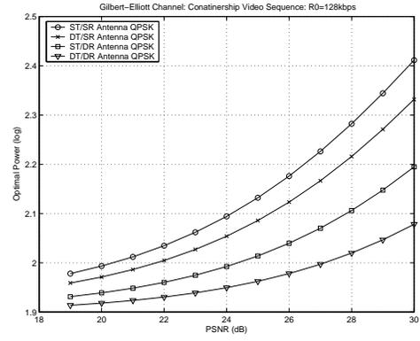
Fig. 7. QPSK plot of optimal power versus peak signal to noise ratio for single/double transmit/receive antenna systems. Containership.qcif video source and the Gilbert-Elliott loss model have been considered.
