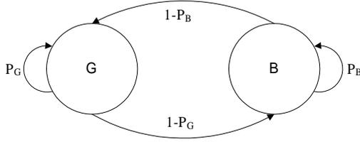
Fig. 2. The two-state Gilbert loss model with the state transition probabilities  $1 - P_G$  and  $1 - P_B$  for  $P_G = \gamma$  and  $P_B = \beta$ . The symbol loss probabilities are specified by  $e_G = 0$  and  $e_B = 1$ .
