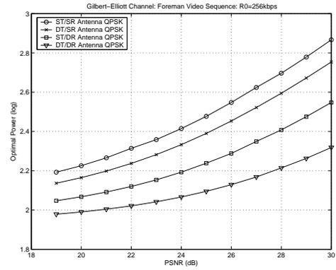
Fig. 8. QPSK plot of optimal power versus peak signal to noise ratio for single/double transmit/receive antenna systems. Foreman.qcif video source and the Gilbert-Elliott loss model have been considered.
