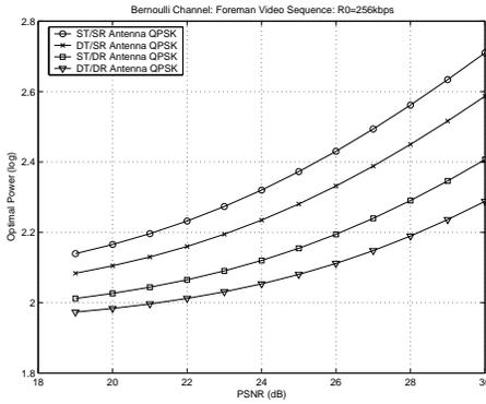
Fig. 6. QPSK plot of optimal power versus peak signal to noise ratio for single/double transmit/receive antenna systems. Foreman.qcif video source and the Bernoulli loss model have been considered.
