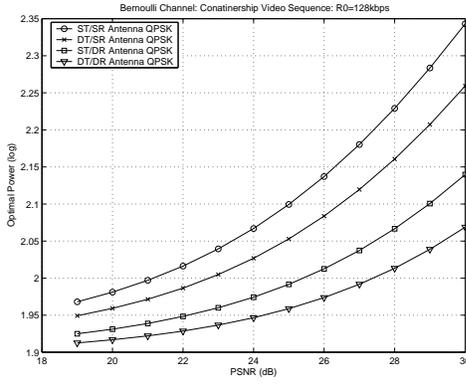
Fig. 5. QPSK plot of optimal power versus peak signal to noise ratio for single/double transmit/receive antenna systems. Containership.qcif video source and the Bernoulli loss model have been considered.
