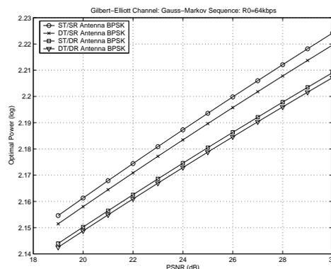
Fig. 4. BPSK plot of optimal power versus peak signal to noise ratio for single/double transmit/receive antenna systems. A Gauss-Markov source with parameter  $\rho = 0.9$  and the Gilbert-Elliott loss model have been considered.
