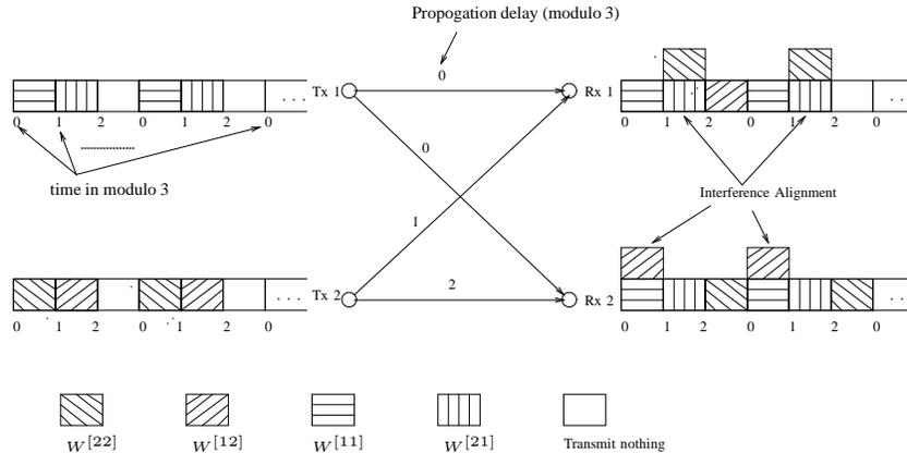
Fig. 3. TDMA scheme achieving  $4/3$  degrees of freedom over the 2 user  $X$  channel with propagation delays
