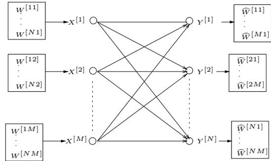
Fig. 1. The  $M \times N$   $X$  network
