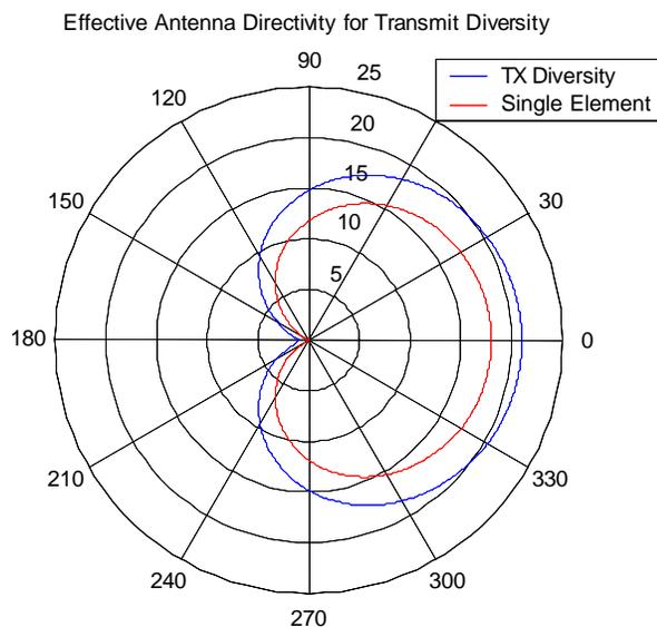
Figure 3: EIRP gain for transmit diversity.
