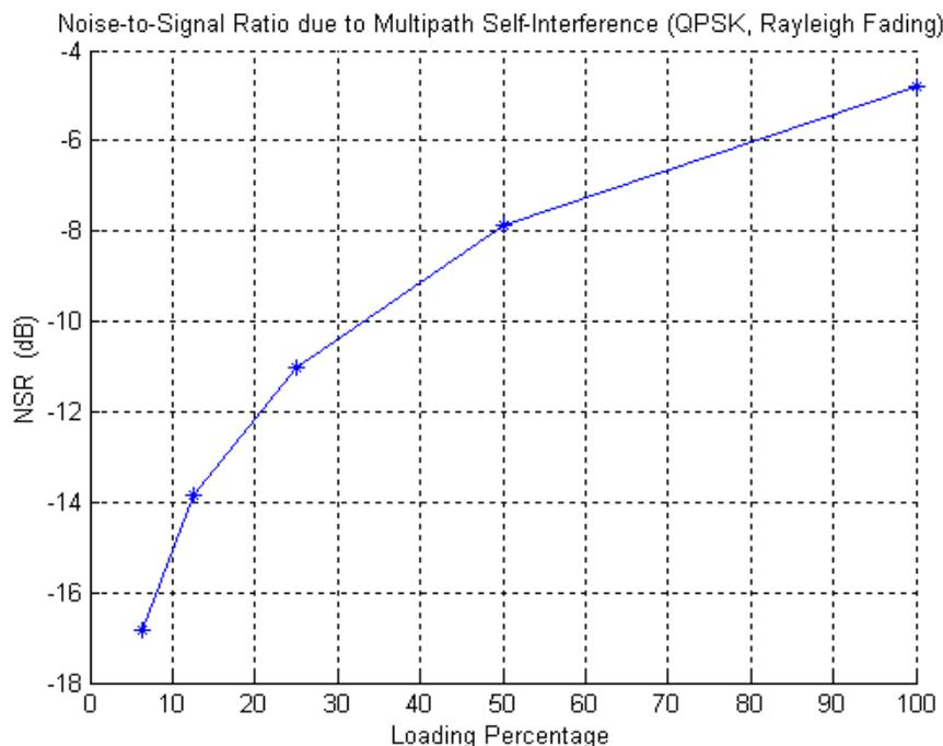
Figure 13: CDMA Noise-to-Signal ratio due to multipath self-interference.
