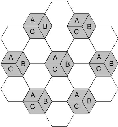
Figure 7: A 3x3 frequency reuse pattern.
