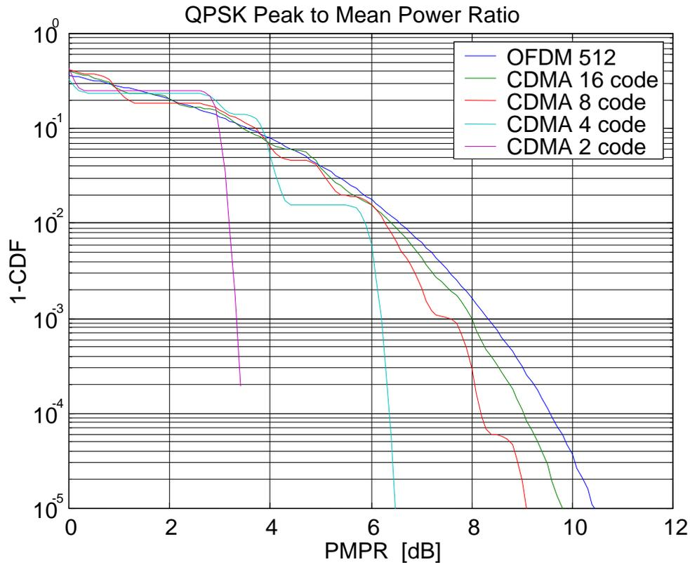
Figure 14: Cumulative distribution of VOFDM and CDMA signal PMPR for spreading factor of 64 and QPSK modulation.
