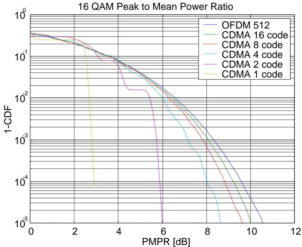
Figure 15: Cumulative distribution of VOFDM and CDMA signal PMPR for spreading factor of 64 and 16QAM modulation.
