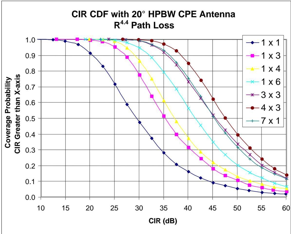
Figure 10: CDF of  $C/I$  with  $20^\circ$  HPBW CPE antenna. The vertical axis corresponds to  $\text{Prob}(CIR \text{ in cell with given reuse configuration} > x\text{-axis})$ .
