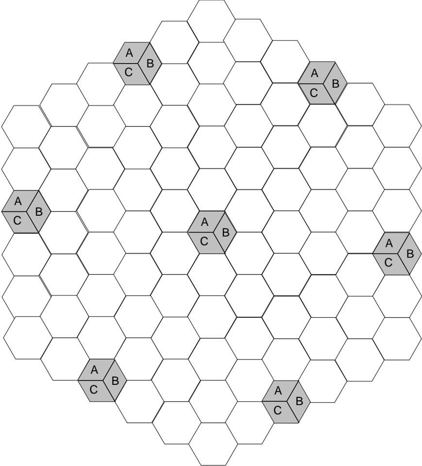
Figure 8: A  $19 \times 3$  frequency reuse pattern.
