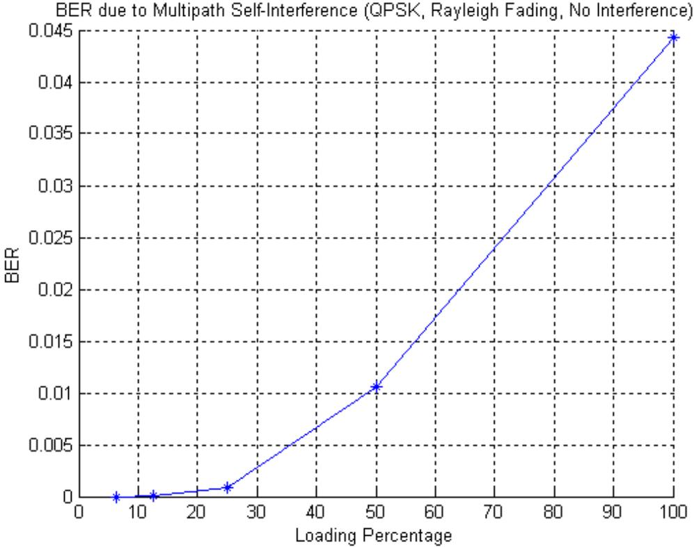
Figure 12: CDMA raw BER due to multipath self-interference.
