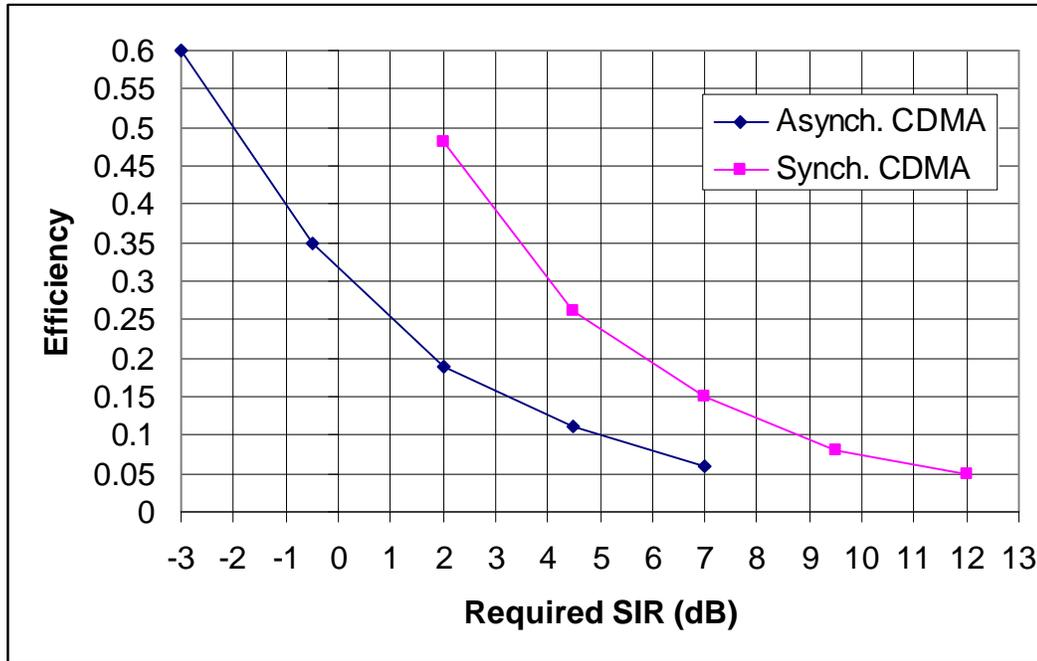
Figure 11: Efficiency of synchronous and asynchronous CDMA system.
