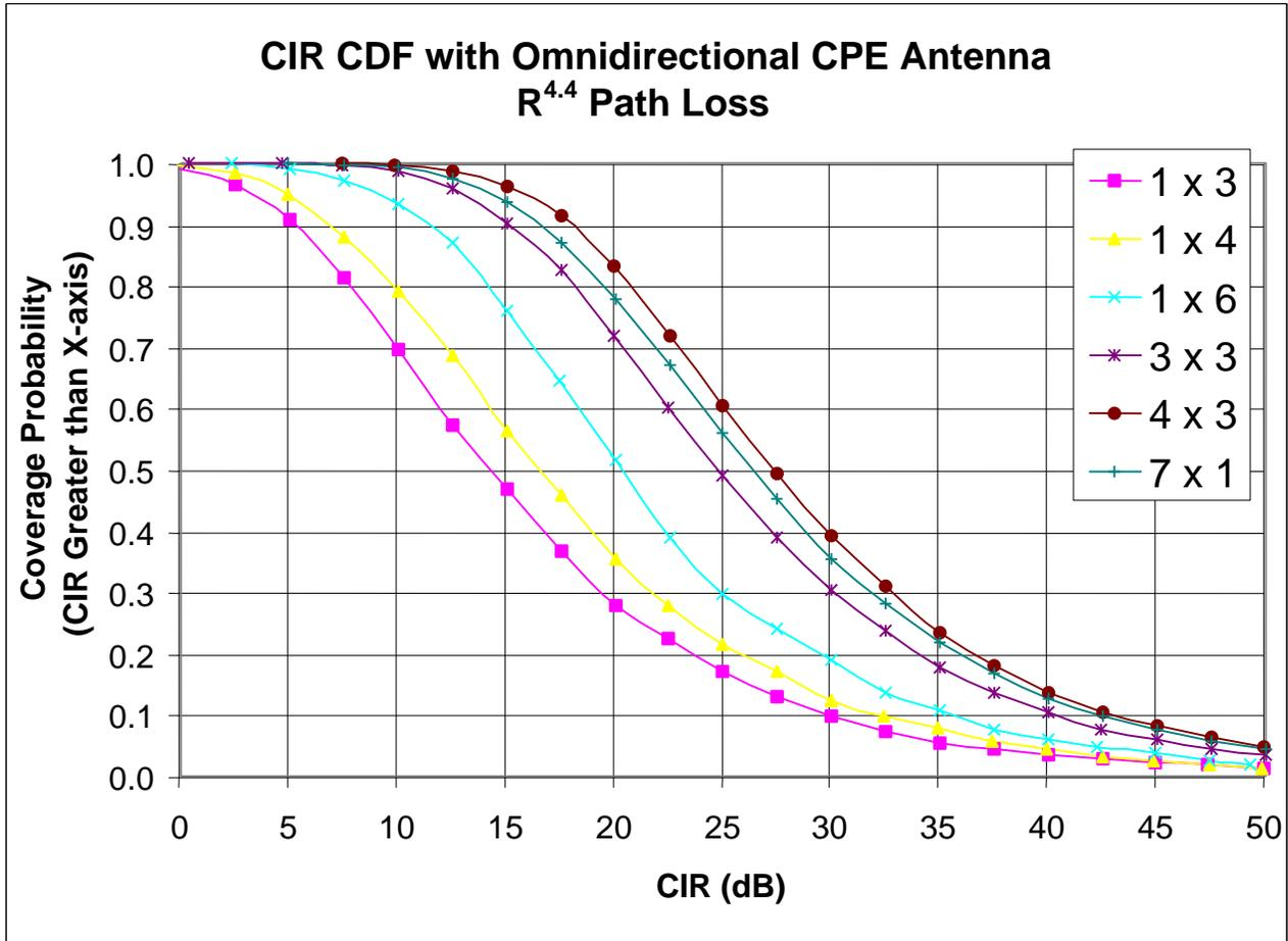
Figure 9: CDF of  $C/I$  with omnidirectional CPE antenna. The vertical axis corresponds to  $\text{Prob}(C/I \text{ in cell with given reuse configuration} > x\text{-axis})$ .
