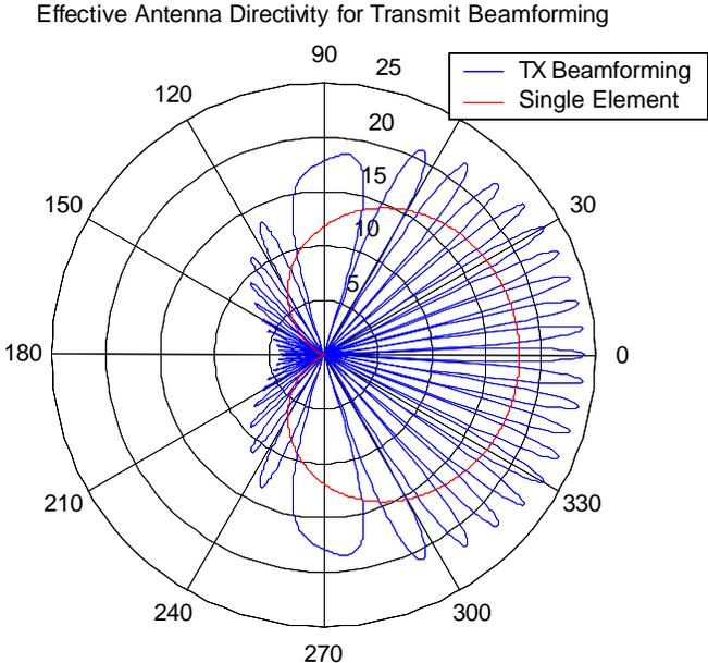
Figure 4: EIRP gain for transmit beamforming.
