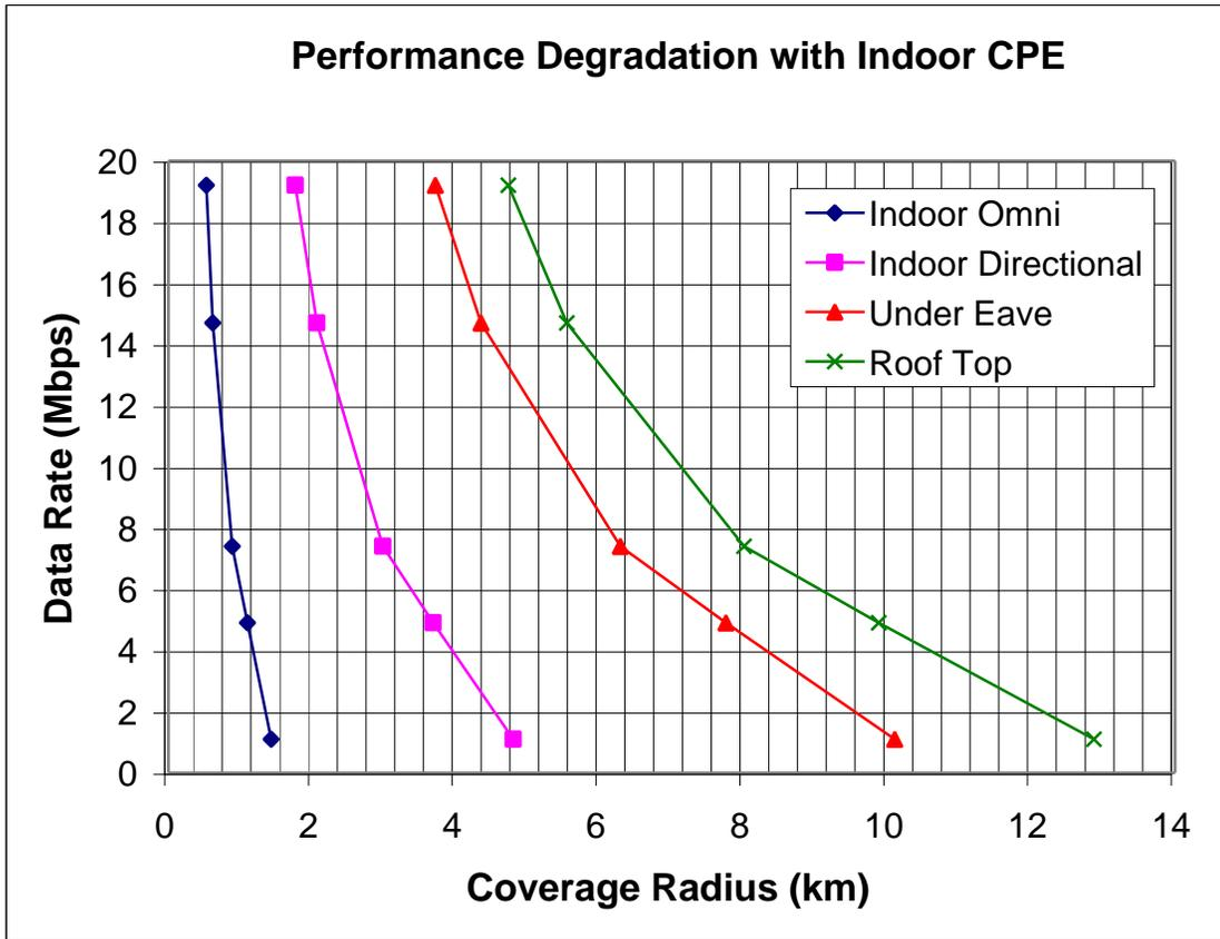
Figure 2: Performance degradation with indoor CPE.
