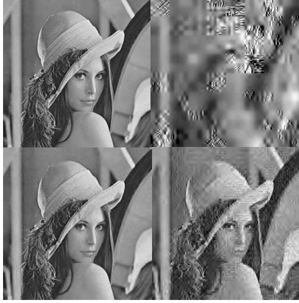
Fig. 9. A comparison of the original and reconstructed sample Lena images utilizing L = 100\text{Bytes} . Clockwise from the top left: the original image, the reconstructed image at SNR_G equal to 6\text{dB} , 9\text{dB} , and 13\text{dB} , respectively.
