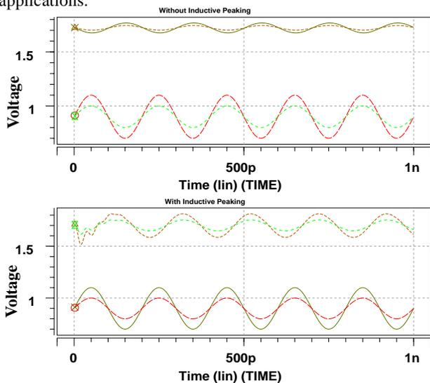
Fig. 9. (a) Input and output waveforms of a CML buffer without inductive peaking. (b) Input and output waveforms of a CML buffer with inductive peaking
