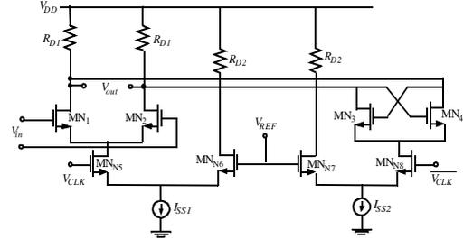
Fig. 7. The circuit schematic of the new CMOS CML latch circuit.
