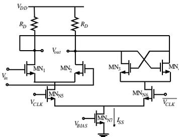
Fig. 6. the circuit schematic of a CMOS CML buffer.
