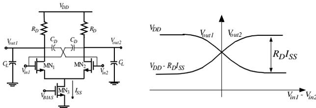
Fig. 1. (a) A neutralized CMOS differential pair. (b) Transfer characteristics.
