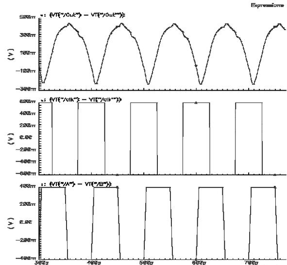
Fig. 11. The 20GHz new CML latch. (a) The input data at 20GHz. (b) The half-rate clock at 10GHz
