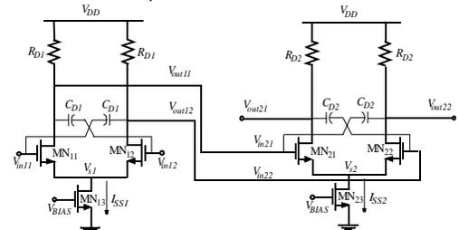
Fig. 2. Two CML buffers in cascade
