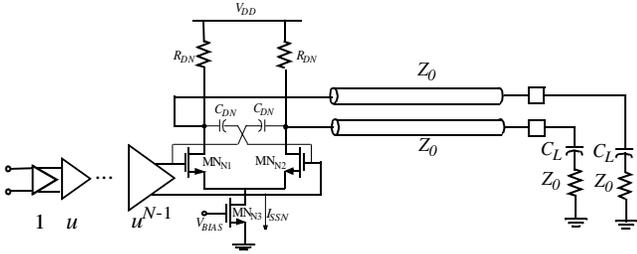
Fig. 3. An output CML buffer driving off-chip loads. The chip-package interface is electrically modeled using a lossless transmission line.
