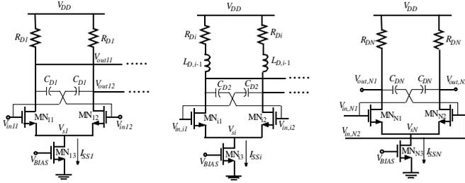
Fig. 5. Multiple stage CML buffers along with the inductive peaking
