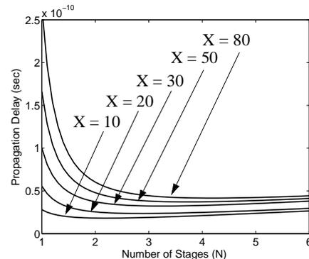
Fig. 8. Delay vs. number of stages for CML tapered buffer chain.
