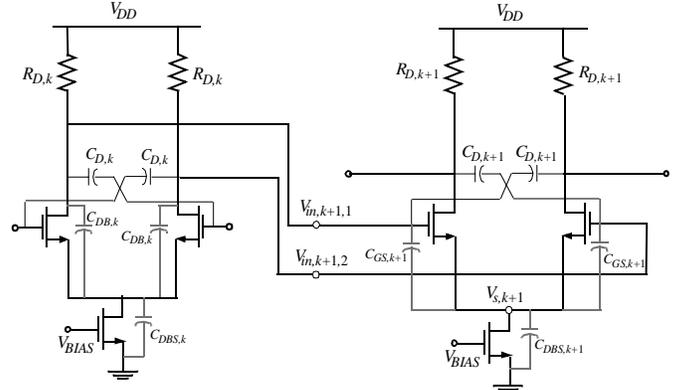
Fig. 4. The  $k^{\text{th}}$  and  $(k+1)^{\text{st}}$  stages of a tapered CML buffer along with the parasitic capacitances
