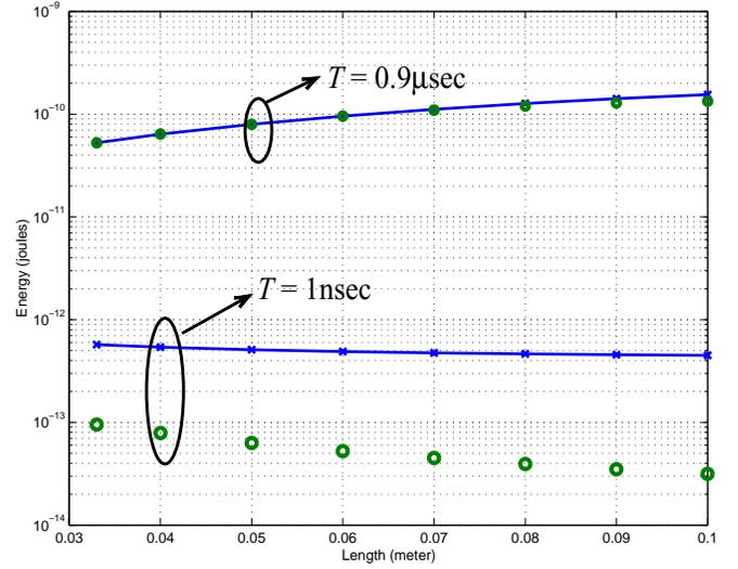
Fig. 6. A comparison between the energy-length variation of the equivalent overdamped RLC- $\pi$  circuit and that of single overdamped RLC circuit modeling a lossy transmission line. The comparison has been made for two values of cycle time,  $T = 1\text{nsec}$  and  $T = 0.9\mu\text{sec}$
