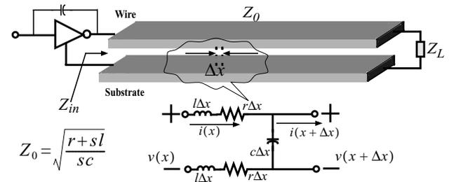
Fig. 1. The schematic of a lossy transmission line along with the circuit representation of a differential length  $\Delta x$
