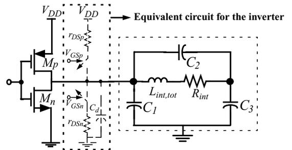
Fig. 4. The equivalent RLC- $\pi$  circuit model of a lossy coupled transmission line driven by a CMOS inverter
