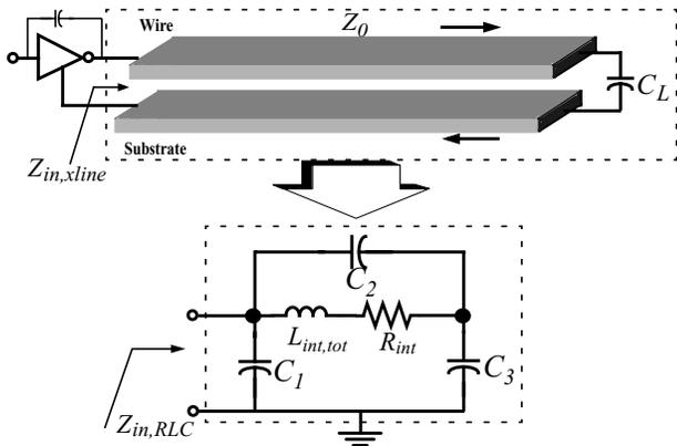
Fig. 2. A lossy transmission line and its equivalent RLC- $\pi$  circuit representation
