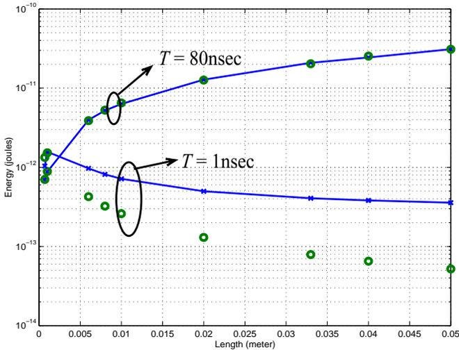
Fig. 5. A comparison between the energy-length variation of the equivalent underdamped RLC- $\pi$  circuit and that of single underdamped RLC circuit of a lossy transmission line. The comparison has been made for two values of cycle time,  $T = 1\text{nsec}$  and  $T = 80\text{nsec}$
