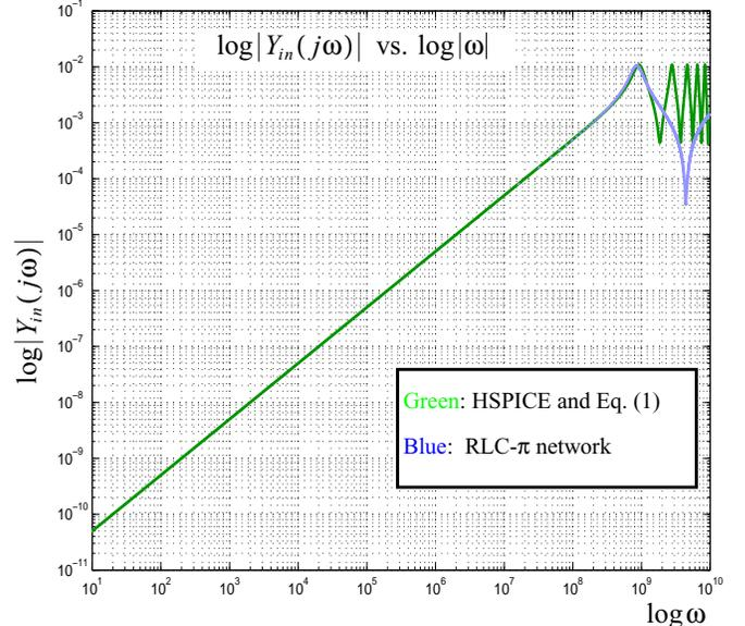
Fig. 3. The magnitude response of the driving point admittance of an electromagnetically coupled lossy transmission line obtained using HSPICE simulation, using the direct simulation of Eq. (1), and by replacing the line with its equivalent RLC- $\pi$  circuit
