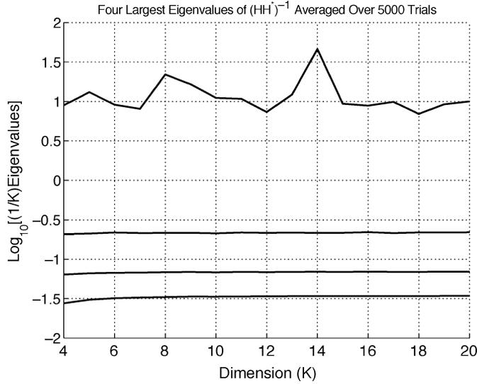
Fig. 1. Numerical comparison of the mean behavior of the four largest eigenvalues of  $(HH^*)^{-1}$  as a function of  $K$ . The figure was generated using 5000 trials, and the eigenvalues are normalized by  $K$ . The largest eigenvalue has an erratic plot because its true mean is infinite (for all  $K$ ), and it is clearly orders of magnitude larger than the remaining eigenvalues.
