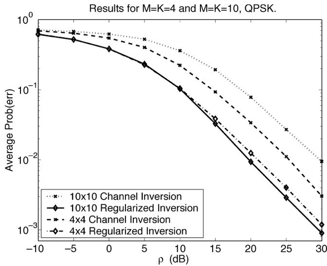
Fig. 3. Comparison of the SEP for plain (8) and regularized (19) channel inversion for  $K = 4$  and  $K = 10$ . The raw error rate as a function of  $K$  worsens for plain channel inversion, but improves (slightly) for regularized inversion.
