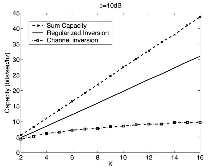
Fig. 4. Comparison of the sum capacity (5) (dashed line) as a function of  $K$  (where  $M = K$ ) for  $\rho = 10$  dB, with the regularized channel-inversion sum rate (32) (solid line) and the plain channel-inversion sum rate (dash-dotted line). Unlike plain channel inversion, regularized inversion has linear growth with  $K$ .
