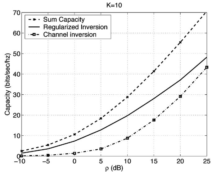
Fig. 5. Comparison of sum capacity (5) (dashed line) as a function of  $\rho$  for  $K = M = 10$ , with the regularized channel-inversion sum rate (32) (solid line) and the plain channel-inversion sum rate (dash-dotted line). At low power, regularized inversion approaches  $C_{\text{sum}}$ , while for high  $\rho$ , it approaches  $C_{\text{ci}}$ .
