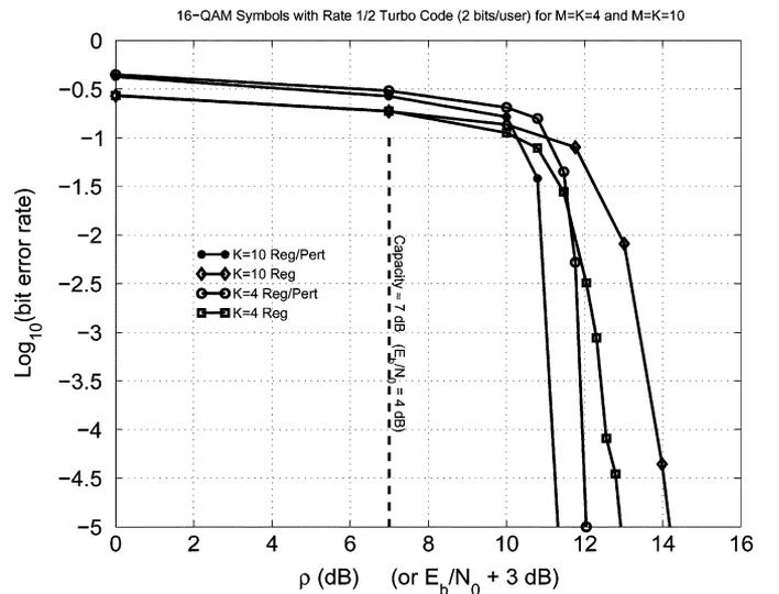
Fig. 5. Bit probability of error for rate  $r = 1/2$  turbo-encoded data using 16-QAM symbols, for  $M = K = 4$  and  $M = K = 10$ . The performance of combining regularization and perturbation is much better than regularization alone; the best performance is obtained for  $M = K = 10$ .
