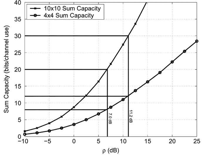
Fig. 3. Sum-capacity for  $M = K = 4$  (lower curve) and  $M = K = 10$  (upper curve) as a function of the receiver additive-noise variance. The marker lines show that to achieve  $C = 8$  ( $K = 4$ ) or  $C = 20$  ( $K = 10$ ), the (reciprocal) noise variance must be  $\rho = 1/\sigma^2 = 7$  dB. For  $C = 12$  ( $K = 4$ ) or  $C = 30$  ( $K = 10$ ), the noise variance must be  $\rho = 11.2$  dB.
