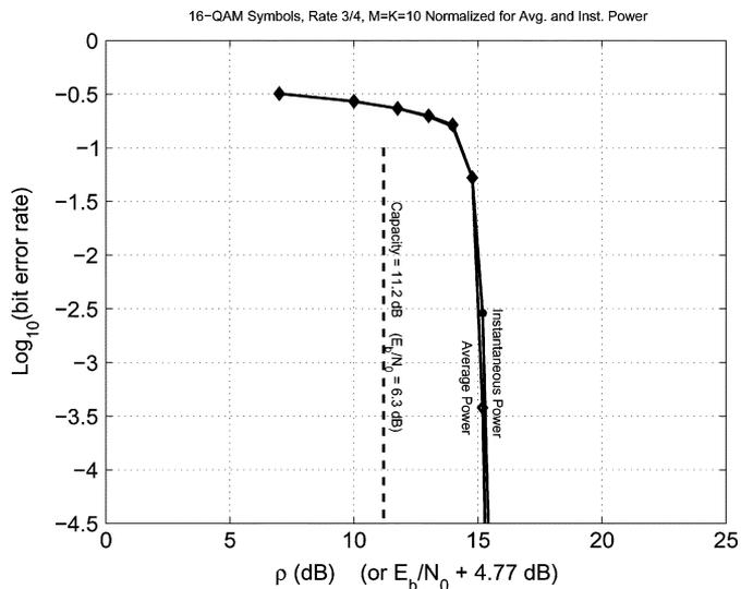
Fig. 6. Bit probability of error for rate  $r = 3/4$  turbo-encoded data using 16-QAM symbols, for  $M = K = 10$ . The curve on the right (instantaneous power constraint) uses normalization at the transmitter by  $\sqrt{\gamma}$ ; the curve on the left (average power constraint) uses normalization by  $\sqrt{E\gamma}$ . The difference in performance is small.
