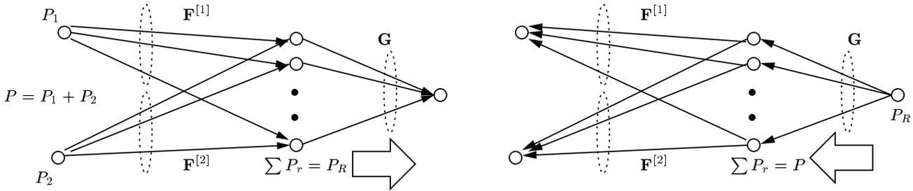
Figure 1: Dual Parallel AF Relay MAC and BC channels
