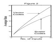
A numerical comparison between scalar and vector coding for Rayleigh fading diagonal MIMO systems is drawn in Figure 2. We notice that the gains with vector coding are significant. The average throughput for 20 inputs at an average transmit SNR of 30 db is about 40% higher for vector coding.
