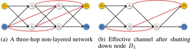
Fig. 5. Interference neutralization exploiting memory
