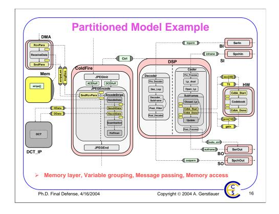
During variable partitioning, a new layer of memory behaviors is inserted, variables are grouped under the memories according to the selected mapping, variable accesses are refined into memory accesses and remaining global variables are distributed into local PE memories and synchronization is updated to exchange updated data values via message passing.
