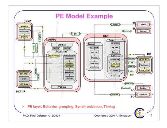
During behavior partitioning, an additional layer of behaviors representing allocated PEs (shown in red) is inserted, original specification behaviors are grouped under PE behaviors according the selected mapping, synchronization behaviors and channels are inserted to preserve execution semantics and leaf behaviors are annotated with estimated execution delays. Not that as a consequence, shared variables become system-global variables between PEs.
