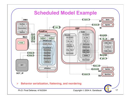
During static scheduling, selected concurrent behaviors are serialized, if necessary parts of the behavior hierarchy are flattened and child behaviors are re-arranged in the selected execution order.
