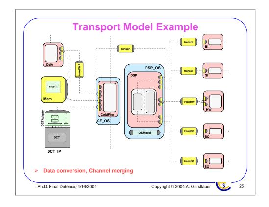
During channel streaming, presentation and session layers are inserted to implement conversion of abstract data types into network bytes and to merge channel into a set of streams between PEs. As part of data conversion, memory behaviors are refined to a byte-accurate representation of their data layout.
