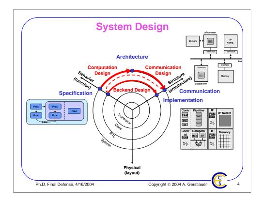
Using the Y-Chart for classification of design processes, design in general is the process of moving from a behavioral to a structural and eventually physical description where designs can be done at different levels of granularity from individual transistors up to complete systems.
