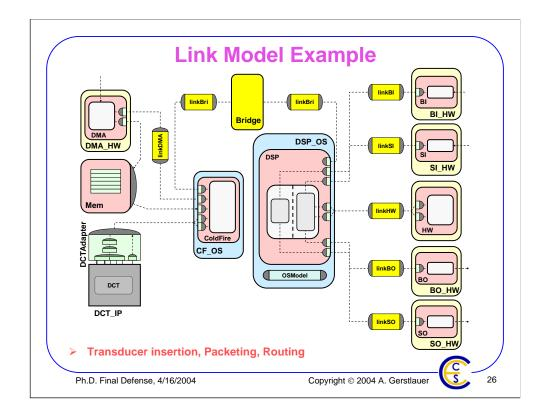
During network segmenting, transducers are inserted to divide and bridge the network into several segments, splitting end-to-end channels into point-to-point links as necessary. Inside PEs and transducers, transport and network layers are inserted to perform the necessary packeting and routing.
