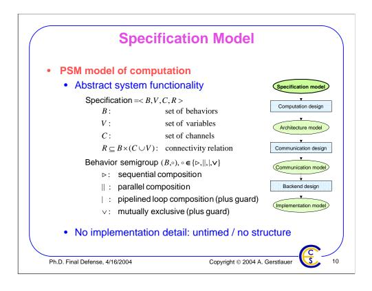
As mentioned previously, the starting point for system design is the system specification model. The specification model is a program state machine model of computation. System functionality is described as a set of behaviors that communicate through variables and abstract channels. Behaviors can be arranged hierarchically in a sequential, parallel, pipelined or state machine fashion. Behaviors the leaf of the hierarchy then contain basic algorithms in the form of C code.
