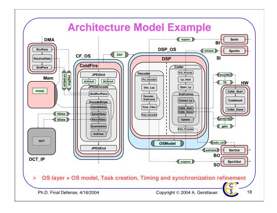
Finally, during dynamic scheduling, an OS layer that includes the selected OS model is inserted around each programmable PE, any remaining concurrent behaviors are turned into OS tasks, and timing and synchronization inside tasks is replaced with corresponding OS model primitives.
