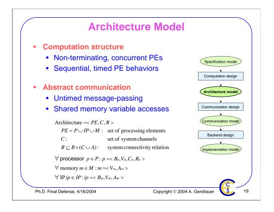
The result of computation design is the architecture model. The architecture model describes the system computation structure as a virtual architecture of non-terminating, concurrent PEs communicating via abstract channels or shared memory accesses. Each PE in turn is described as a set of local behaviors connected by local variables and channels.
