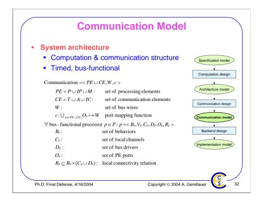
The result of communication design is the communication model. It is a busfunctional, timing-accurate description of the complete computation and communication system architecture. The communication model is a netlist of processing and communication elements connected via bus wires. Each busfunctional component in turn is described as a set of local behaviors, variables, channels, bus drivers and ports.
