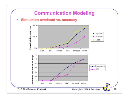
Benefits and trade-offs in terms of model complexities vs. model accuracies for communication models at different levels of abstraction are shown here. The graphs show simulation runtimes on a logarithmic scale and communication delays measured by setting computation delays to zero and normalized against the communication delay in the final implementation.
