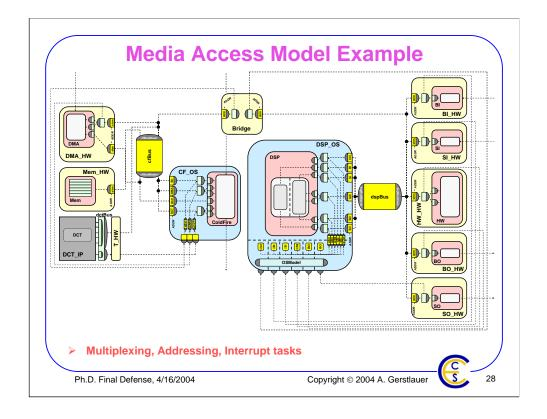
In the second step of link grouping, data streams in each segment are then multiplexed over a shared medium channel. Stream layers that perform the necessary media addressing are inserted into the components. In addition, interrupt tasks that communicate with bus drivers through semaphores are inserted to implement control transactions.
