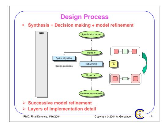
Each of the different design tasks is then further broken down into several successive design steps. With each step, a design model at a certain level of abstraction is synthesized into a model at the next lower level. The result is a flow with successive refinement of design models where a new layer of implementation detail is added to the design in each step.
