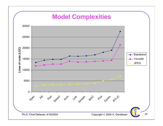
Model complexities as measure by the number of lines of code for models of different designs at different levels are shown here. As expected, models generally grow linearly with lower levels of abstraction. At the RTL level, however, model sizes grow exponentially due to the high overhead necessary for cycle-accurate state machine modeling where growth depends to a large extend on the size of the hardware part.
