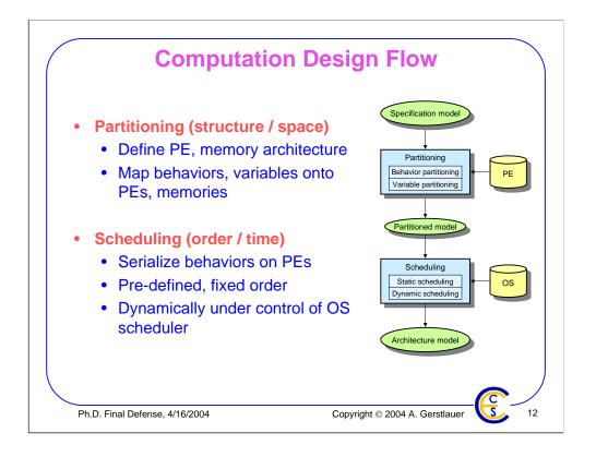
The purpose of computation design is to implement the computation in the specification as represented by its behaviors operating on variables on a virtual architecture of processing elements and memories.
