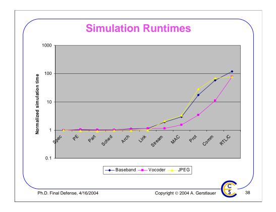
In terms of simulation overhead, it can be seen that all throughout computation design, almost no additional overhead is introduced. Only in the link design phase, simulation runtimes start growing exponentially as explained earlier during communication modeling. Again, exponential growth of runtimes during backend design depends exclusively on the relative size of the hardware part in the design.
