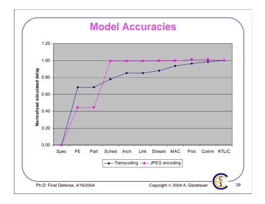
Finally, looking at accuracies of models at different levels of abstraction, results confirm the choice of the architecture model as intermediate model for exploration, especially considering the fact that no additional simulation overhead is introduced up to this point. For the designs shown here, the architecture model is over 80% accurate. PE and partitioned models are generally not accurate enough as they ignore the effects of sequential execution on PEs.
