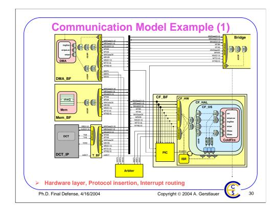
Finally, timing-accurate bus-protocol implementations are inlined into the system components, exposing the underlying bus wires. For programmable PEs, hardware models are inserted that accurately describe the PE's interrupt handling behavior. Finally, bus-functional arbiter and interrupt controller models are inserted and connected.
