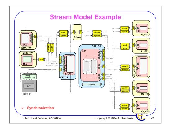
As a first step of link grouping, links are split into separate control and data streams based on the type of bus interface of each link. Link layers that implement synchronization over control channels around each data transaction are inserted.
