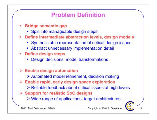
In general, the semantic gap between specification and implementation is too big to be completed in one step. In order to bridge the gap, the design process therefore has to be broken down into smaller, manageable steps.
