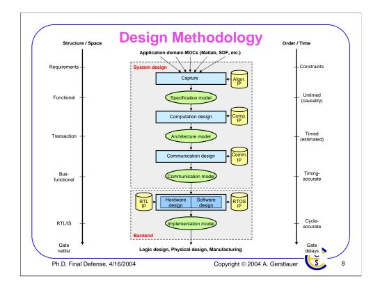
The overall design methodology is shown here. In general, as we move down in the level of abstraction from specification to implementation, more and more implementation detail in the form of structure and order is added.
