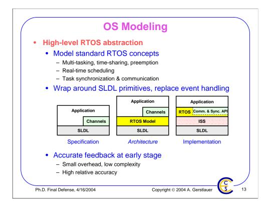
In order to properly model dynamic scheduling behavior at this high-level of abstraction, an abstracted model of the underlying RTOS is inserted into the design. The RTOS model describes expected RTOS behavior at a high-level without unnecessary implementation details. It supports all the standard RTOS concepts for multi-tasking, dynamic real-time scheduling including preemption and inter-task communication and synchronization.
