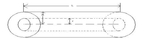
Figure 1: Hollow cylinder (pipe) with inner radius r, outer radius R and length L.
