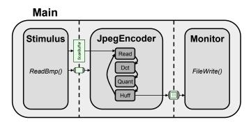
The Stimulus is connected to the JpegEncoder through a shared ScanBuffer variable representing the CCD sensor array. In addition, a c\_handshake channel represents the signal that the camera shutter has been triggered and that encoding of the CCD sensor picture should be started. At the other end, the Monitor receives a stream of encoded bytes from the Huffman encoder (Huffencode) through a c\_queue representing the file I/O interface.
