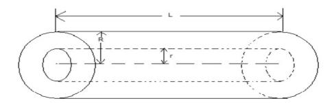
Figure 1: Hollow cylinder (pipe) with inner radius r, outer radius R and length L.
