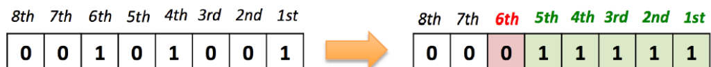
(a) Posterize the least 6 significant bits of the red channel for pixel(0,0)
