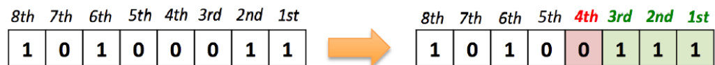
(c) Posterize the least 4 significant bits of the blue channel for pixel(0,0)
