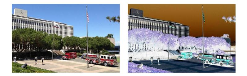
Subtract R[x][y], B[x][y] and G[x][y] from 255 and set the new value back.
