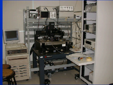
Probe station for RF circuits characterization
